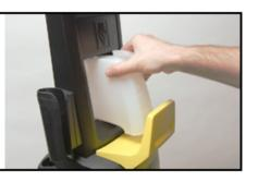
Attach detergent tube on back side of handle, pull through handle, and attach filter. You're ready to add detergent!
